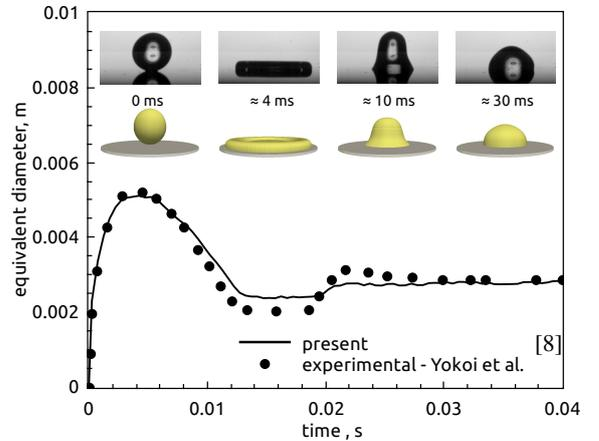
Figure 4: Comparison of predicted (present) equivalent diameter against Yokoi et al. [8]
