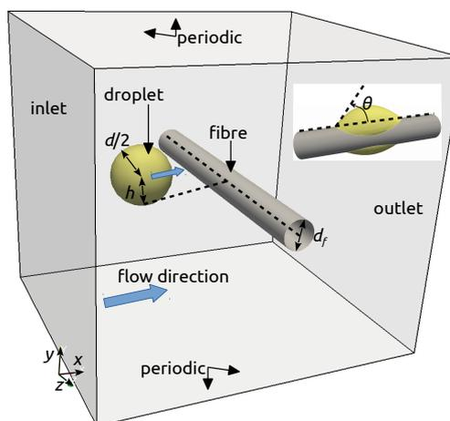
Figure 1: Schematic of the geometry and computational domain
