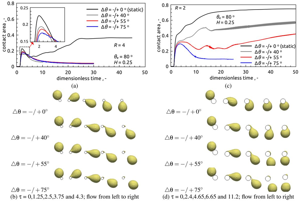
Figure 5: Influence of contact angle hysteresis on the interaction between an impacting oil mist droplet and fibre
