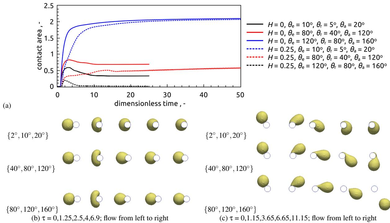
Figure 6: Influence of contact angle on the interaction between an impacting oil mist droplet and fibre; the angles represent  $\{\theta_r, \theta_e, \theta_a\}$
