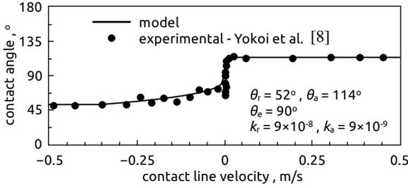
Figure 2: Dynamic contact angle model from Yokoi et al. [8]
