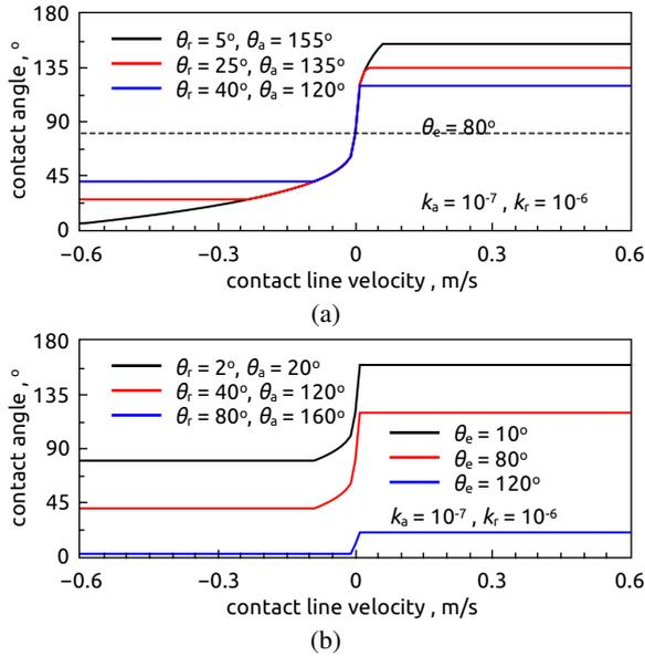
Figure 3: Dynamic contact angle models used for the study
